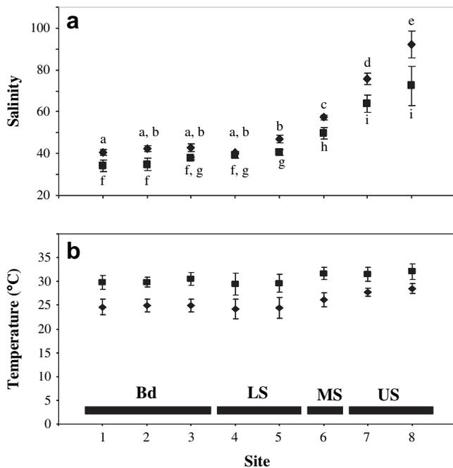
**Fig. 3.** Spatial variations (mean  $\pm$  SE) of salinity (a) and temperature (b) in the Sine Saloum estuary from April 2007 to March 2008. Bandiala channel (Bd); lower (LS), middle (MS) and upper (US) sections of the Saloum. Lozenges correspond to dry/cold and squares to wet/hot seasons respectively. Means with different letters are significantly different at  $P < 0.05$  (Nemenyi test).
